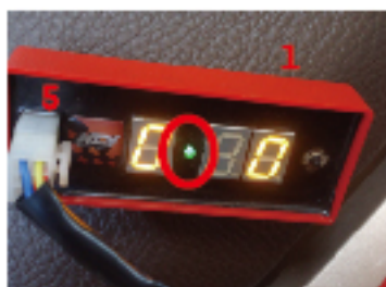
9. CONNECT NCY WIRE TO ADJUSTER AND TURN ON SWITCH TO CHECK WHETHER ADJUSTER SHOWS SIGN OR NOT.
