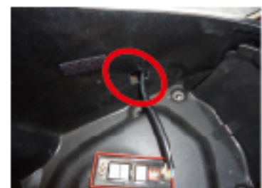
11. PIERCE A HOLE IN THE LUGGAGE BOX TO MAKE WIRE PASS THROUGH.
