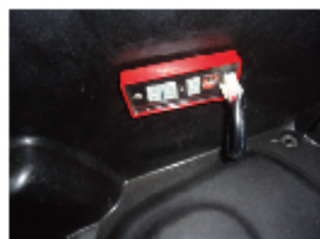
12. USE THE VELCRO TO ATTACH ADJUSTER IN THE LUGGAGE BOX. THIS ADJUSTER IS NOT WATERPROOF.
