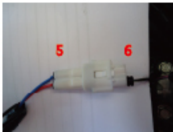
7. INSERT THE WIRE (+) INTO NO.6 CONNECTOR [CONNECT TO NO.5 CONNECTOR (RED)].
