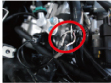
2. CUT INJECTOR WIRE SET.
