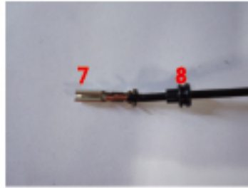
3. INSERT WATERPROOF PLUG AND PIN INTO THE CUT WIRE (STEP 2).
