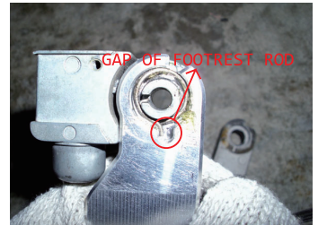
8. ROTATE THE RAISING POINT OF ROTATING SPRING INTO THE GAP OF FOOTREST ROD..
