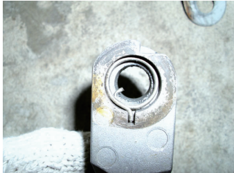
5. REMOVE ROTATING SPRING FROM ORIGINAL FOOTREST ROD. (NOTICE THE INSTALLING DIRECTION OF ROTATING SPRING AS REMOVING)
