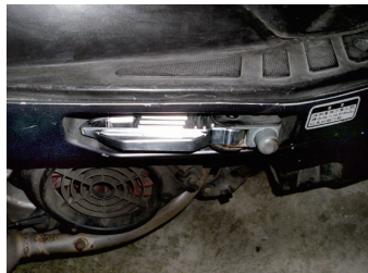
11. IF THE FOOTREST ROD SET WORKS NORMALLY, INSTALL IT ON THE SCOOTER DIRECTLY.
