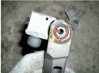
4. PRESS THE SHAFT OF THE BASE. SEPERATE THE BASE AND THE FOOTREST ROD.
