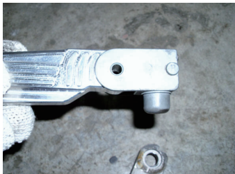
10. CHECK IF THE MOVEMENT OF THE FOOTREST ROD SET WORKS NORMALLY OR NOT. IF NOT, PLEASE FOLLOW STEP 6 AND INSTALL AGAIN.
