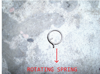
5. REMOVE ROTATING SPRING FROM ORIGINAL FOOTREST ROD. (NOTICE THE INSTALLING DIRECTION OF ROTATING SPRING AS REMOVING)
