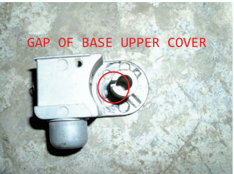
7. PUT THE RAISING POINT OF ROTATION SPRING INTO THE GAP OF BASE UPPER COVER.
