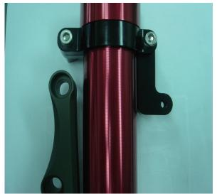
1.LOOSE THE FRONT FORKS RING SCEWS, ADJUST THE RING INTO THE SUITABLE ANGLE AND FASTEN THEM AGAIN.
